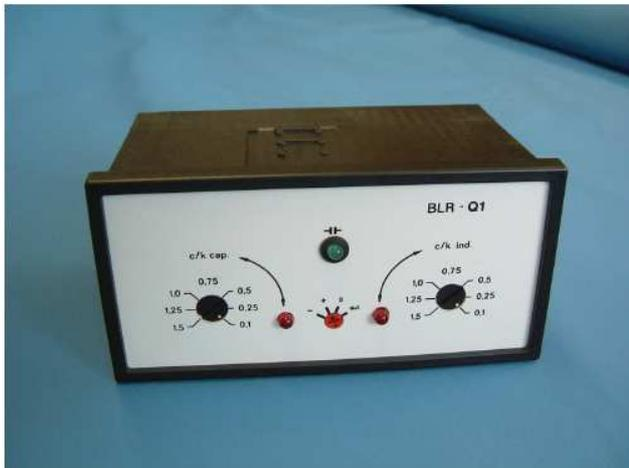
This single step relay facia size 144 x 72mm allows the user to set independent lead/lag threshold reactive currents. It has hand/auto/off control available on the relay. This controller is well suited to HV Capacitor installations on overhead lines or on any switchboard HV or LV.
